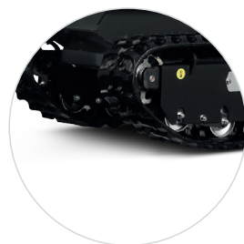
C — Tendicingolo a grasso Greased track tensioner
